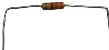
Figure 3. Bending legs on a resistor.
